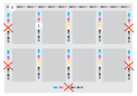
Illustration 4: Placement of the "S" and "L" version on sheets with long cut-off pages. The red X marks unsuitable positioning.
